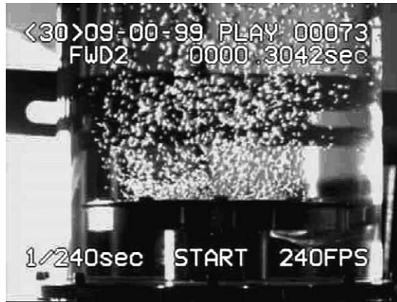
Fig. 7. Air-bubbles detaching from porous plate in dispersion box.
